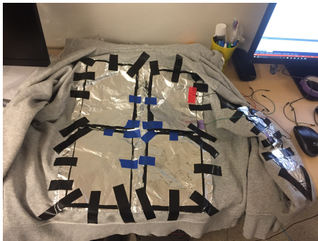
Figure 2: Design of sensory shirt: contains a shirt with 8 pressure sensors that uses velostat to measure the pressure and aluminium foil to make the sensors conductive
