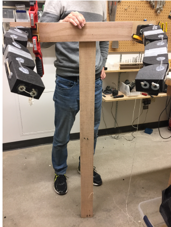
Figure 5: The T-shape structure used for making the backbone of HugBot
