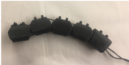
Figure 3: Prototype of a 3D printed arm with 3 joints and a fixed part on which the other joints rest
